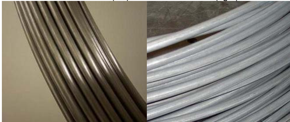
Note the dull, mottled appearance of the stabilized material.
