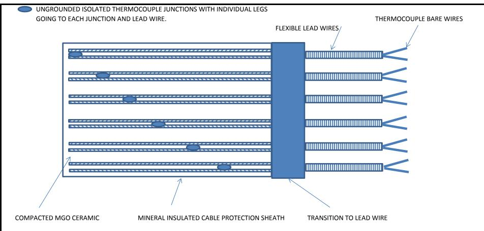
AVAILABLE IN K, J, E, N, CALIBRATIONS AND 304, 316, 310, 321, 347, I600 SHEATH MATERIALS. MULTIPOINT OVER ALL LENGTHS ARE ONLY LIMITED BY THE AVAILABLE MI CABLE. THE POCKET JUNCTION THERMOCOUPLE USES OFF THE SHELF MINERAL INSULATED CABLE THAT HAS A DIAGONAL WIRE LAY OUT.
