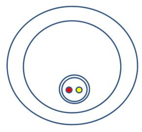
Conventional design multipoint that is not fully filled. Note: The thermocouples at the end may not be in contact with the sheath which will slow down the response time. This type multipoint should only be used in an application where measuring temperature change is not critical to the operation.
