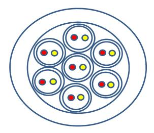
Example of a fully filled seven point multipoint thermocouple. cross section showing all of the MI cables.
