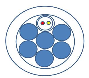
Cross section showing six filler wires and one remaining MI cable.
